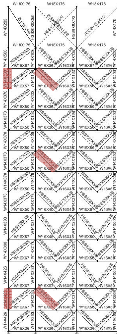
Figure 9 – Analyzed members of the lateral force-resisting system
